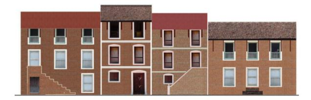
Computer rendering of a proposed restoration employing traditional building style and materials. The roof will be covered with red-painted corrugated steel as seen in the images on the right.
